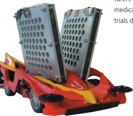
An electric motor-driven miniature car powered by a direct methanol fuel-cell battery utilizing pore-filling electrolyte membranes
