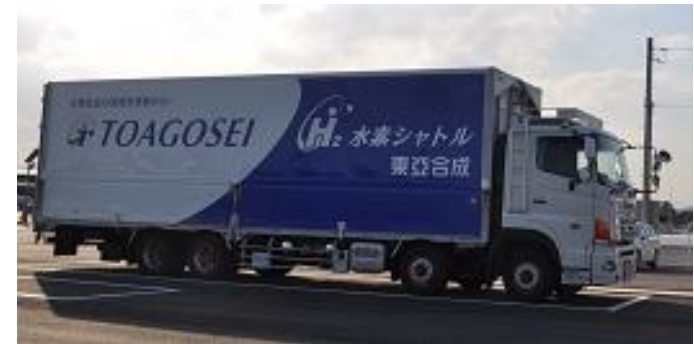
Mobile hydrogen station
